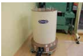
Compact NDA system incorporating a helium-3 substitute ceramic scintillator
